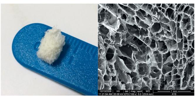
Figure 1 Macroscopic (left) and cross-section microscopic view obtained by scanning electron microscopy (SEM) (right) of a collagen based scaffold material
