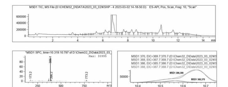
Fig. 5. LC/MS-spectrum 3-(2-bromo-4-fluorophenyl)-4-ethyl-5-(hexylthio)-4H-1,2,4-triazole 2f
