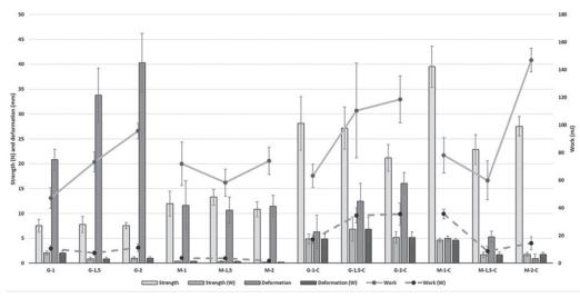
Fig. 4. Comparison of tested parameters observed through tensile testing (strength, work, deformation) in dry and wet states (W)
