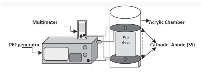
Fig. 2. The PEF generator scheme
