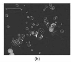
Fig. 2. Optical microscope images of mirtazapine-loaded PLGA microparticles, bars correspond to  $1000 \mu m$ : (a) A, (b) E-M600
