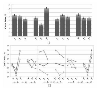
Fig. 3. Effects of the factor levels on the mean values of Carr's index: I – main factor effects, II – effects of paired interactions
