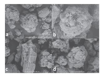
Fig. 2. Fluid-bed granulated CPE a) Advantol® 300, b) Ludipress® LCE, c) Smartex® QD 50, d) Smartex® QD 100
