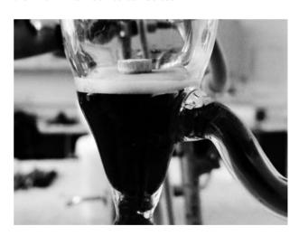
Fig. 1. Water absorption rate test of tablet
