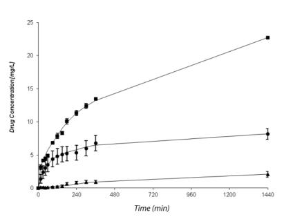
Fig. 5. Dissolution profile of diclofenac sodium release from sample DS-LH-CHC in  $\bullet$  purified water;  $\blacksquare$  McIlvaine's buffer pH 6.8; and  $\blacktriangle$  McIlvaine's buffer pH 3.2 Note: drug concentration of 26.14 mg.l $^{-1}$   $\sim$  100% drug release
