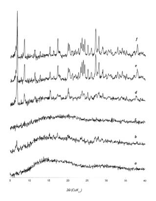
Fig. 3. XRPD spectra of (a) Eudragit® RS PO, (b) 1:9 (w/w) DS/ERS physical mixture, (c) 1:9 (w/w) DS/ERS co-evaporate, (d) DS/ERS 1:1 (w/w) co-evaporate, (e) diclofenac sodium-evaporate from methanol and (f) diclofenac sodium raw
