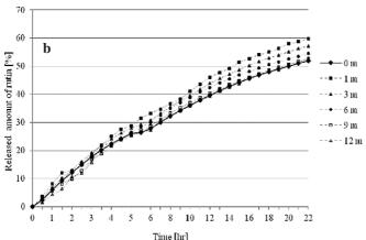
Fig. 5 Rutin dissolution profiles under stability conditions 30/65: (a) final buffer pH 4.0; (b) final buffer pH 6.0
