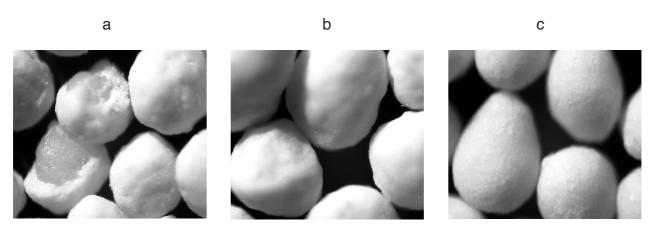
Fig. 2. Sample 1 (a), sample 3 (b) and sample 6 (c) after friability test under condition 200/10/20 (magnification 25x)
