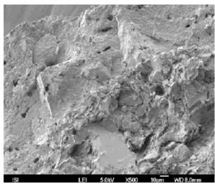
Fig. 3. The cross-section of the layered pellet (left) containing the MCC and LM/ MCC (right) as observed under the scanning electron microscope (magnification  $500\times$ )
