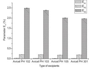
Fig 4. Parameters  $E_{\rm Al\cdot 3}$  in the excipients under study (all columns displayed means of n=20 with 1s error bars)
