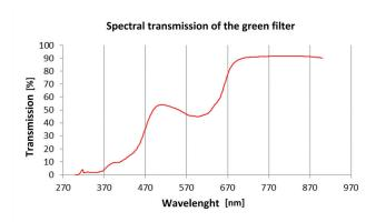
Fig. 1: Spectral characteristics of green chromagen filter.
