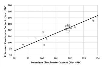
Fig. 4. Regression plots of the comparison between HPLC and UPLC for amoxicillin (a) and potassium clavulanate (a) by the Passing-Bablok method
