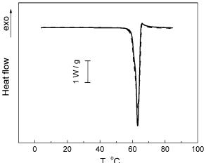
T, °C Fig. 6. Normalized DSC thermograms of TA melting: individual TA (solid line); mixture TA: PH 2: 1 (w/w) (dashed line)
