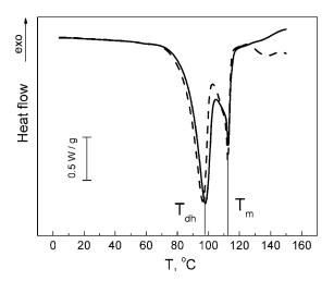
Fig. 8. Normalized DSC thermograms of MgSt (solid line) and MgSt: MgLac (dashed line). The vertical lines indicate the dehydration temperature  $(T_{\rm nh})$  and the melting temperature  $(T_{\rm nr})$  of MgSt.
