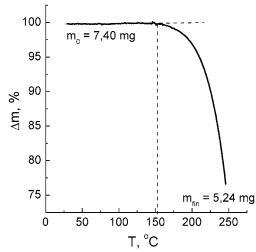
Fig. 5. TGA curve of TA sample. The dotted lines are plotted to show the limit of thermal stability of the TA. The values of initial and final sample mass ( $m_0$  and  $m_{\rm fin}$ , respectively) are indicated.
