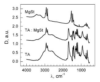
Fig. 3. FTIR spectra of MgSt, TA and their mixtures 20 : 1 (w/w)
