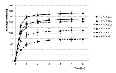
Fig. 1. The swelling profiles of 3% Cu<sup>2+</sup>/alginate particles in phosphate buffer pH = 6.0
