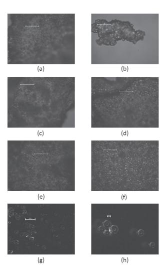
Fig. 1. Picture of optical microscope analysis (a) - E0.1-200, (b) - E1-200, (c) - E0.1-400, (d) - E1-400, (e) - E0.1-600, (f) - E1-600, (g) (h) - R; bar corresponds to 10  $\mu$ m (a, b, c, d, e, f) 500  $\mu$ m (g) and 100  $\mu$ m, respectively (h)
