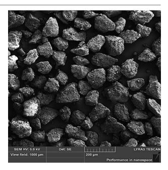
Figure 1. SEM picture of sorbitol particles
