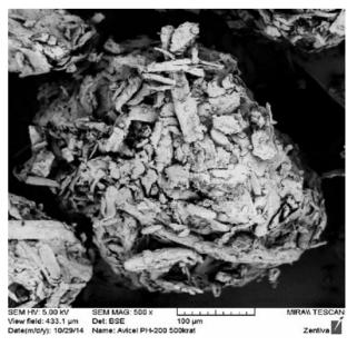
Fig. 1. SEM image of Avicel PH-200 particle, magnification
