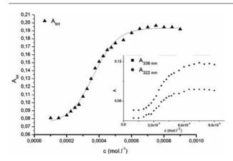
Fig. 3. The dependence of the sum of absorbances of main pyrene peaks  $A_{\rm tot}$  vs. concentration of studied compound (c) 1182-RM-12-14 in 0.1M ethanol solution Inset: Dependence of absorbances (A) of pyrene peaks (322 nm a 336 nm) vs. concentration
