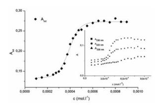
Fig. 2. The dependence of the sum of absorbances of the main pyrene peaks Atot vs. concentration of studied compound (c) 1182-RM-12-14 in water solution
