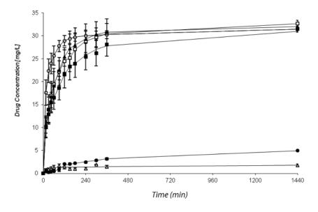
Fig. 2. Dissolution profile of diclofenac sodium release from sample DS/PVP-LH in  $\bigcirc$  purified water;  $\square$  McIlvaine's buffer pH 6.8;  $\triangle$  McIlvaine's buffer pH 3.2; and sample DS/ERS-LH in  $\blacktriangle$  purified water;  $\blacksquare$  McIlvaine's buffer pH 6.8;  $\bullet$  McIlvaine's buffer pH 3.2 Note: drug concentration of 30.74 mg.l $^{-1}$  (DS/PVP-LH) and 32.74 mg.l $^{-1}$  (DS/ERS-LH)  $\sim$  100% drug release
