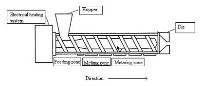
Fig. 1. Single screw extruder (modified from 17)
