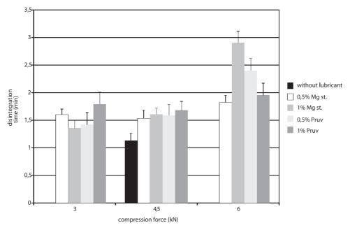
Fig. 4. Disintegration time in function of compression force: Sorbitab SD 250  $\,$
