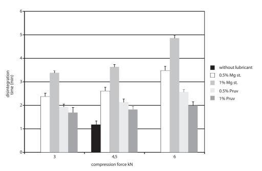
Fig. 5. Disintegration time in function of compression force: Sorbitab SD 500
