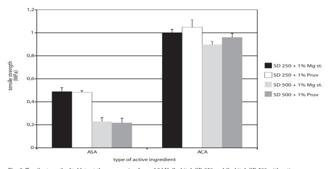
Fig. 6. Tensile strength of tablets at the compression force of 6 kN: Sorbitab SD 250 and Sorbitab SD 500 with active ingredients
