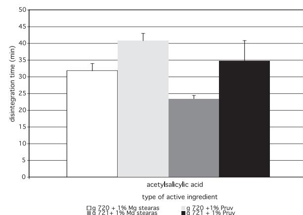
Fig. 7. Disintegration time of tablets at the compression force of 10 kN: galen IQ 720 and 721 with acetylsalicylic acid
