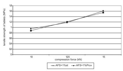
Fig. 1. Tensile strength of tablets in function of compression force: Advantose FS 95 with lubricants
