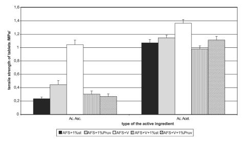
$\textit{Fig. 7. Tensile strength of tablets at the compression force of 12.5 kN. Advantose FS~95 and its \textit{mixture with Vivapur 102 with active ingredients} \\$
